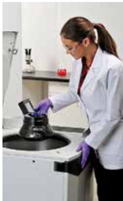
1. Place rotor into the centrifuge chamber
