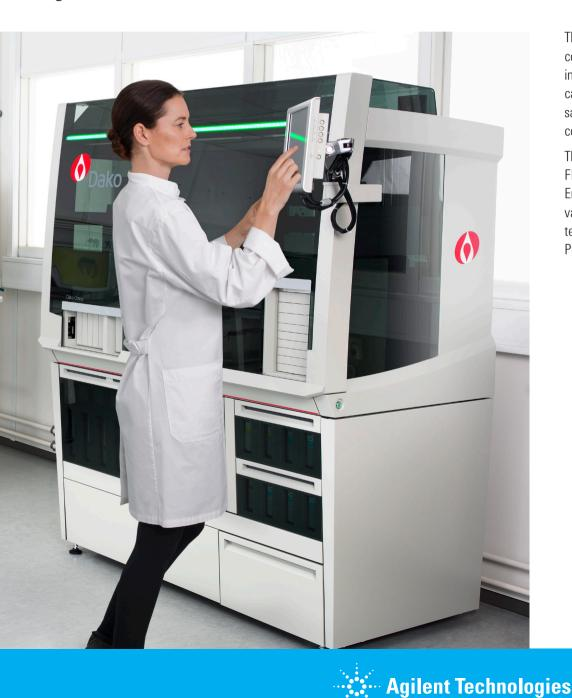
The Dako Omnis solution enables a continuous patient-based workflow, in which IHC, IF and ISH slides can run simultaneously on the same instrument, each with unique combination of antibodies.
