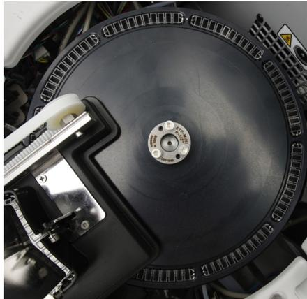
Temperature controlled incubator for 90 cuvette cells. Cuvettes are disposable, so there is no need for extra rinsing to prevent carry-over.
